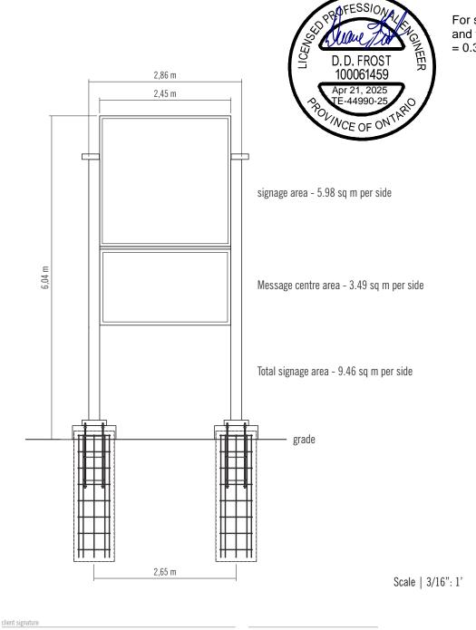
For structural design of columns, base, and footing. Design wind load g(1/50) = 0.36 kPa.
